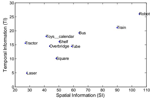
Figure 2. The distribution of content complexity of source video contents. The SI and TI are calculated according to ITU-T P.910.
