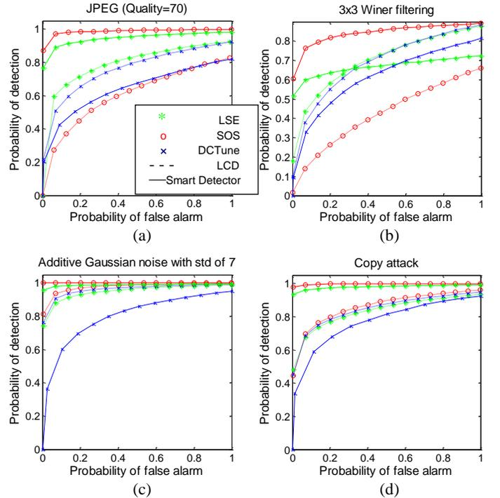
Fig. 8. ROC curves for the 7527  $40 \times 40$  StirMark image blocks after (a) JPEG compression with the quality factor being 70, (b) Wiener filtering with window size being 3, (c) additive Gaussian noise with std of 7, and (d) copy attack.
