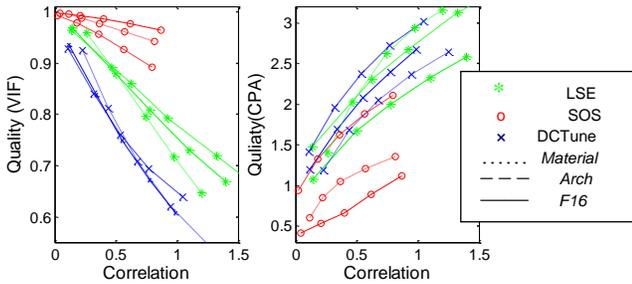
Fig. 5. Curves of the quality of the image embedded with the three types of watermarks versus the correlation after Wiener filtering attack (window size is 3).
